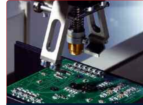
High speed pick and place capability
